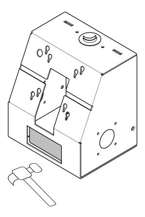
Knock out the micro joint with the hammer
